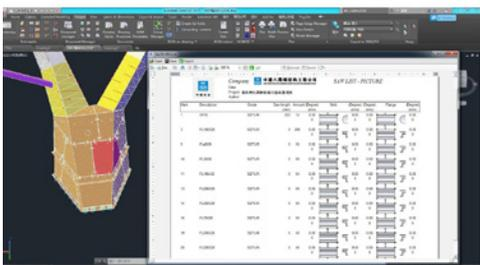
process user-friendly. Section shape of components is inserted by default, improving visibility with engineers and facilitating BIM-based quantity calculation.
