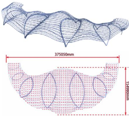
(2) Designed to provide 2D and 3D double-curved support, the support arches are trapezoidal across, tapering off toward the far end. Their internal reinforcement plates make modeling even more difficult;
