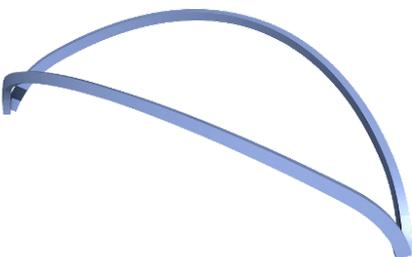
(3) It's difficult to ensure precision processing of the double-curved components. Assembly and welding have to be sequenced to ensure the accessibility and strength of welding. Meanwhile, contracting and deformation caused by welding must be mitigated to deliver the designed shape and specification of the whole structure.
